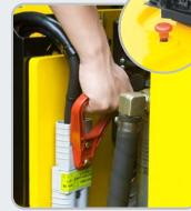
**Battery Disconnect Lever** / Switch
