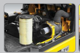
**Easy change air cleaner** The air filter is readily accessible for cleaning or replacement. (7inch Cyclone Type)
