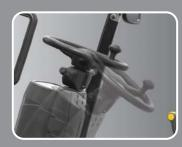
Adjustable steering wheel Steering wheel with horn button can be adjusted by a lever on the right-hand side for the most
